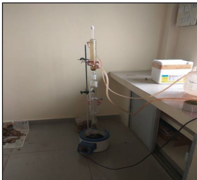
Fig. 3: Extraction process using soxhlet apparatus.
